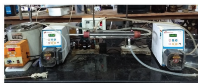
Fig.1: [a] Schematic of Double pipe Heat Exchanger [b] Double pipe Heat Exchanger set up
